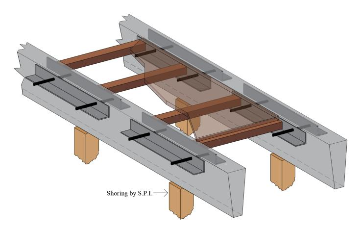
As noted, the joist support the deck formwork, with less shoring than a cast-in-place or posttensioned structure, this speeds up the construction schedule while providing long spans with cost competitiveness. The reshores to the deck below are also minimal, thereby providing access.
