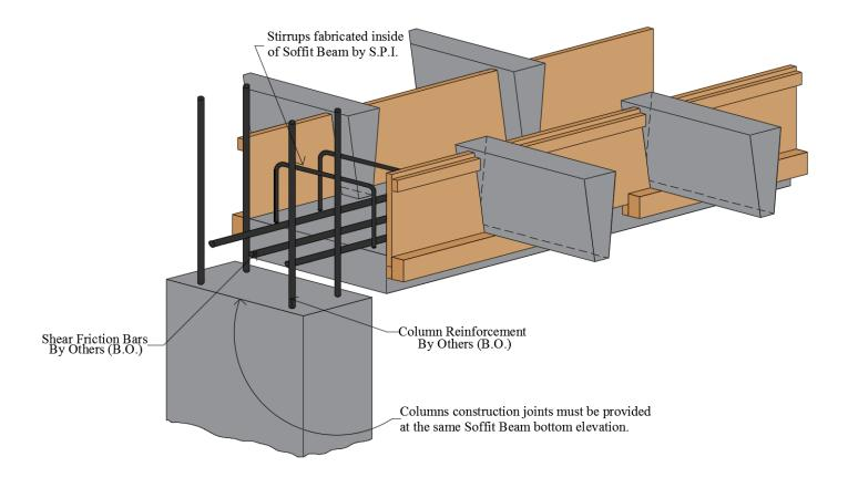
Just like a cast in place beam the soffit beam is poured with the column providing continuity between the beam, and the slab. Beam Stirrups are cast into the Soffit Beam by S.P.I. and the longitudinal reinforcing is placed on the field by others.
